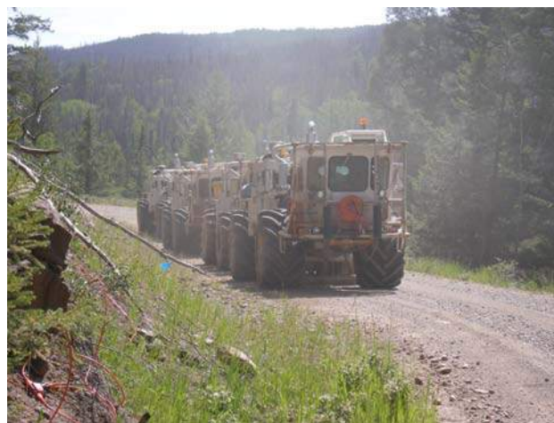
Figure 3. CGGVeritas vibrators shaking on July 2, 2008 on line 5, with dust rising from the base plates.
