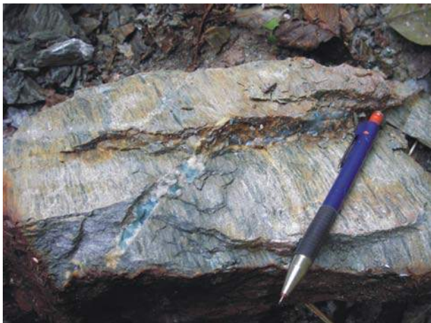
Figure 21. Intensely silica+sericite+carbonate-altered mafic schist with quartz-carbonate and blue-green gypsum veins; in places, quartz-carbonate veins contain blebs of chalcopyrite.
