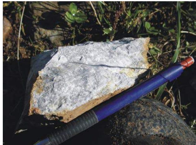
Figure 22. Bleached, highly sericite+silica+fuchsite-altered mafic volcanic rock with up to 4% pyrite mineralization as disseminations, stringers and blebs up to 2 cm in size.
