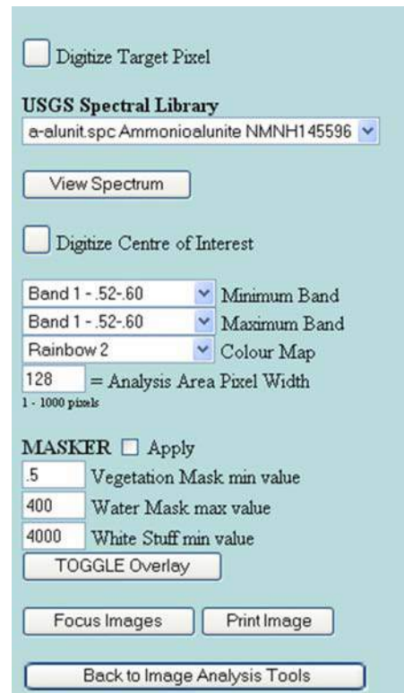
Figure 10. New layout of the 'Spectral Angle Mapper' panel. The 420 entries in the USGS Mineral Spectral Library are available through the pull-down selection box. The 'View Spectrum' button produces a spectrum plot of the selected spectrum.
