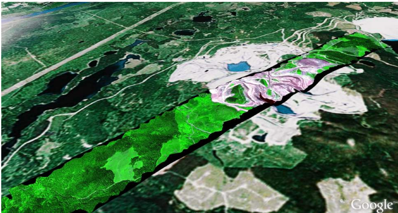
Figure 4. Gibraltar hyperspectral false-colour image draped over Google™ Earth terrain. The hyperspectral image is a mosaic constructed from the three individual lines flown over this site.
