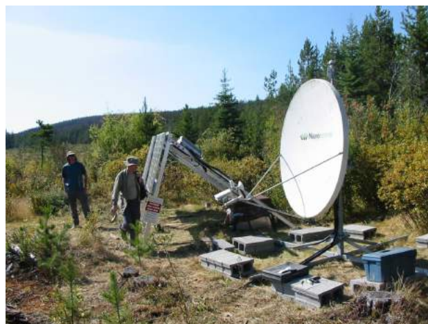
Figure 3. Photograph of Nechako seismic station RAMB, showing the typical station layout, with solar panels and satellite dish (seismic vault is not visible).
