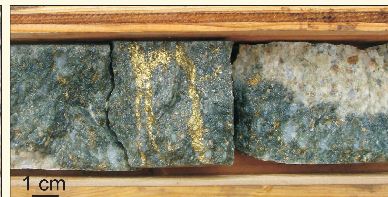
Intense green mica alteration and associated chalcopyrite mineralization overprinting the Bethsaida granodiorite.
