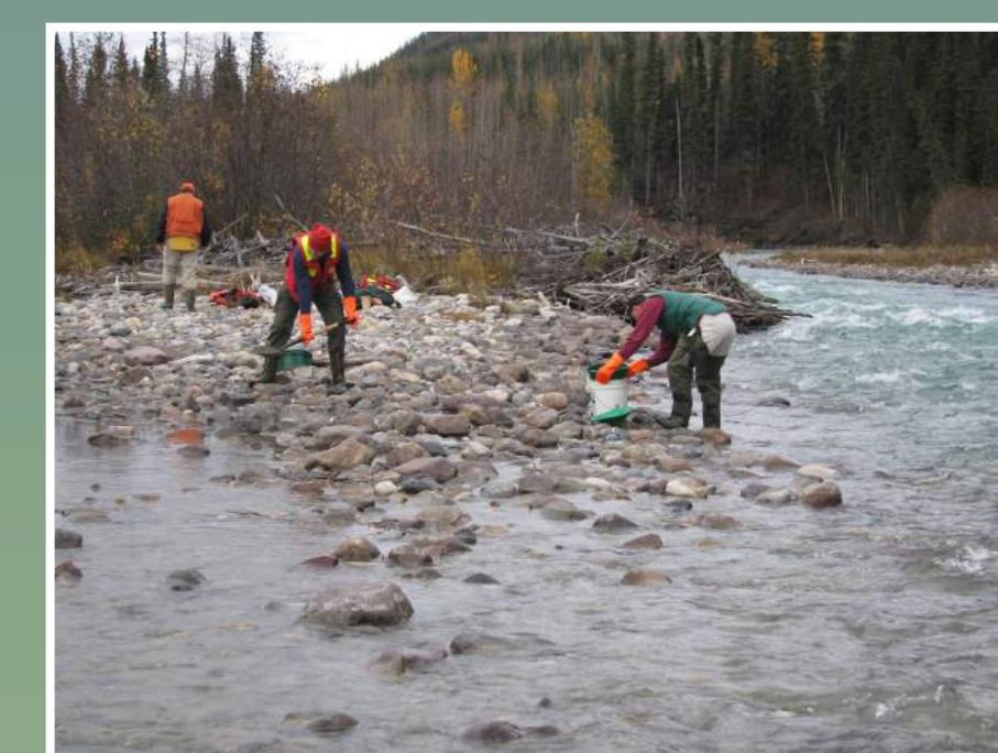
GSC employees Steve Adcock, Alain Grenier and Martin McCurdy collect a bulk sediment sample from a site along the Alaska Highway in northeast British Columbia (contributed by S. Day, GSC).
