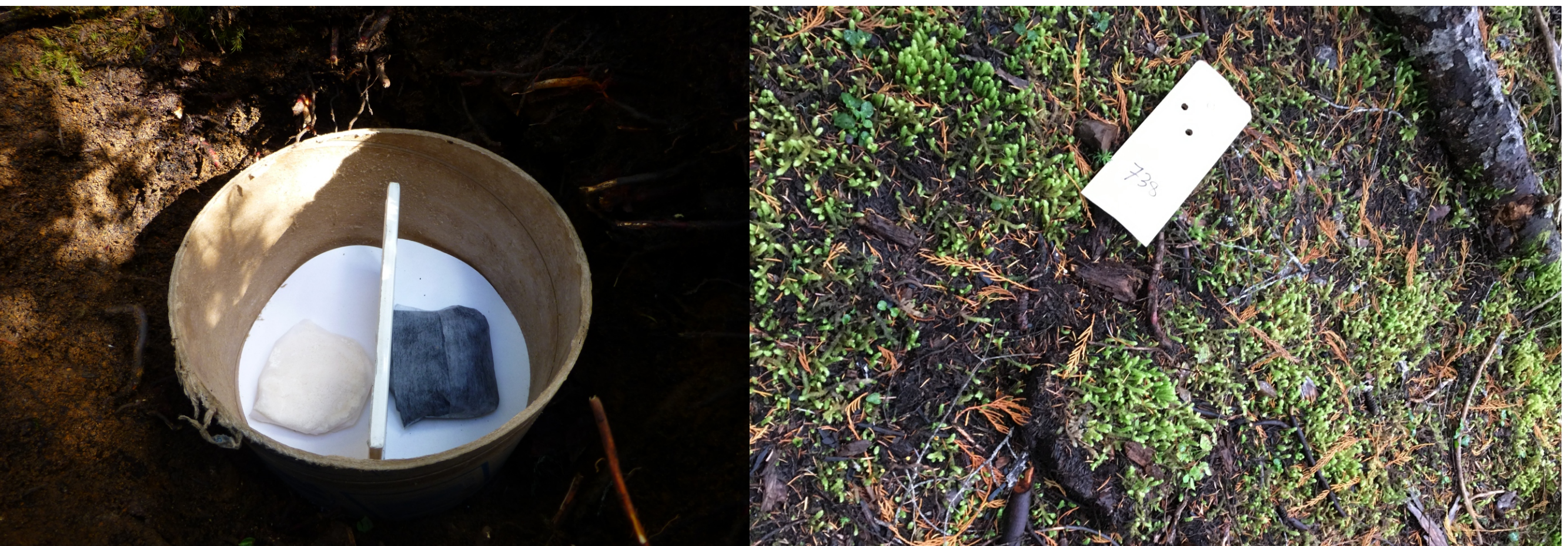
Ion collection device with ion exchange resin. An example of a buried ion collector site. (left) and activated charcoal sachets (right). Sachets are separated by a ceramic tile to prevent cross contamination. Tube diameter: 19mm.
