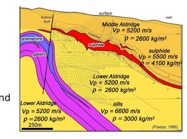
**Figure II-B.** Model of seismic response from the Sullivan deposit.
