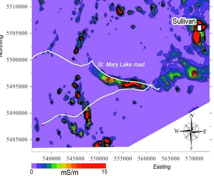
Result: By combining stratigraphy and structure from subsurface data (e.g., seismic) with electrical conductivity, zones with metals may be targeted.
