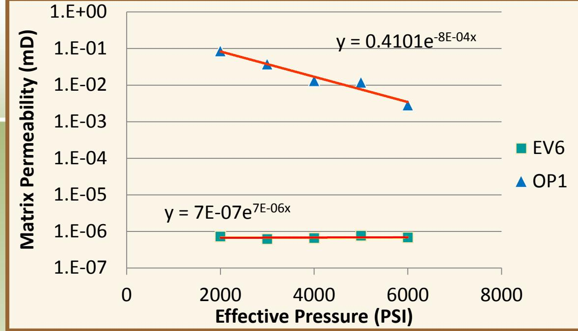
EV6: isotropic, carbonate rich, less sensitive
