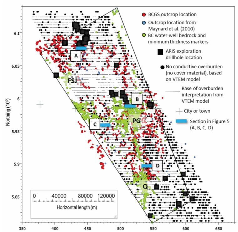
Constraining data used for overburden-thickness modelling. Constraining data from VTEM inversion models are derived from interpretations digitized along line on east-west VTEM lines spaced 4 km apart. Project area lies within the black quadrilateral. Abbreviations: PG, Prince George; FSJ, Fort St. James; Q, Quesnel.
