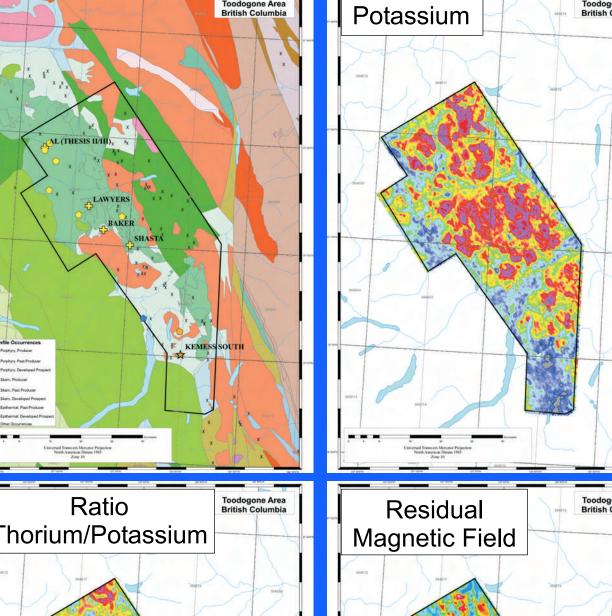
In the Iron Mask batholith area (Afton) virtually all known porphyry-related mineralization produces diagnostic airborne survey signatures, appearing as equivalent thorium/potassium ratio lows combined with relative total field positive anomalies. Separately, neither technique
