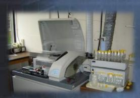
ICPMS AND INAA METHODS CAN PROVIDE OVER 70 ELEMENT DETERMINATIONS
