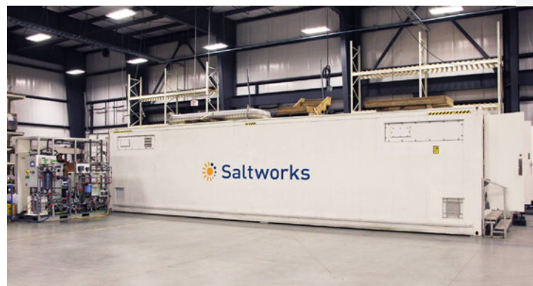
↑ The Saltworks AirBreather Pilot project has been testing a process that harnesses waste heat from natural gas production to treat saline wastewater. Photo: Saltworks Technologies
