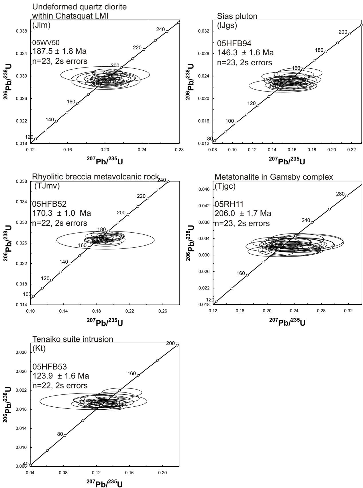
Figure 4. Standard concordia diagrams with U-Pb zircon data by laser ablation ICP-MS plotted at the 2σ confidence level; all interpreted ages are based on weighted averages of  $^{206}\text{Pb}/^{238}\text{U}$  dates, also reported with 2σ errors; see text for discussion.
