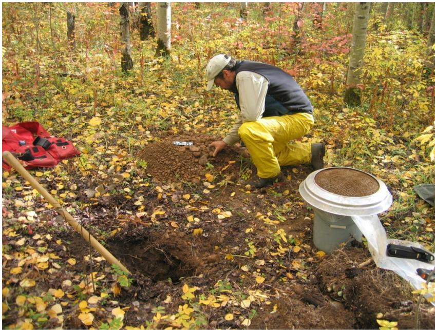
Figure 3: Glacial sediment sampling in support of kimberlite exploration in northeastern BC. Photo courtesy of I.R. Smith.
