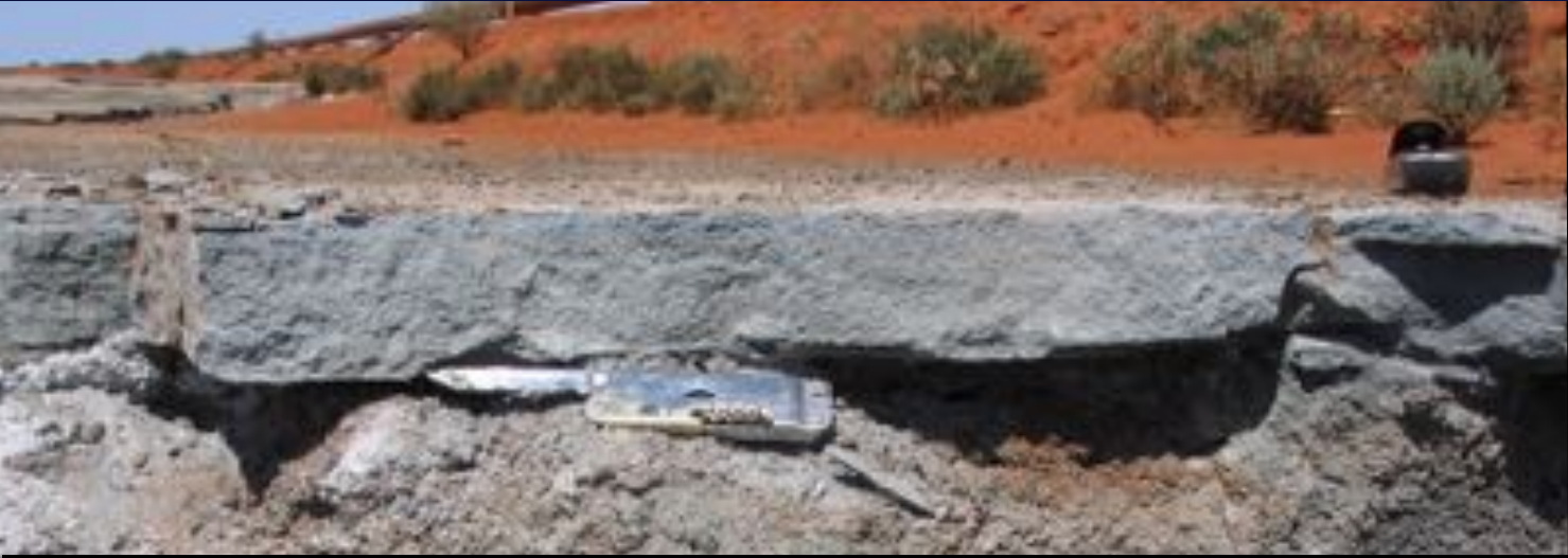
Cementation of tailings originally deposited as water-sand slurry Mt Keith Nickel Mine, WA, Australia
