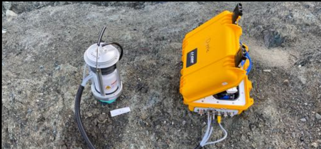
CO 2 direct air capture measured with soil gas chambers 3 kg CO 2 / m 2 / year
