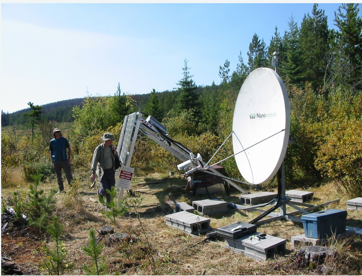
Photograph of Nechako seismic station RAMB, showing the typical station layout, with solar panels and a satellite dish (seismic vault is not visible).
