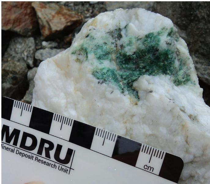
**Figure 9:** Quartz vein material with green fuchsite mica replacement of wallrock fragment, with sulphide minerals. Such K-bearing alteration material, where occurring with visible gold, are considered as best representatives of the timing of gold mineralization.
