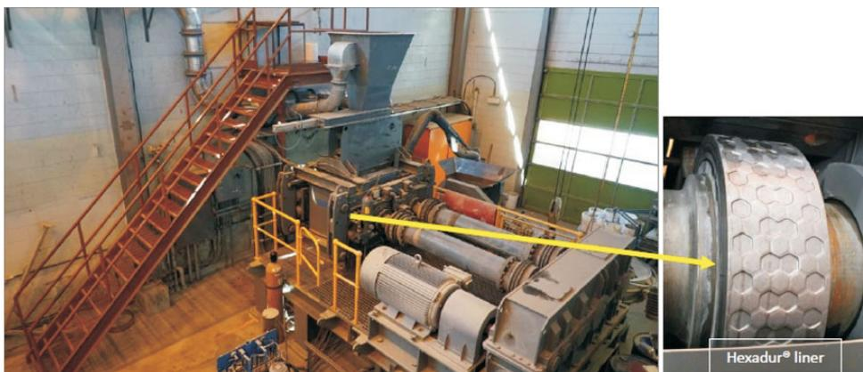
**Figure 1.** Photos of the Köppern pilot-scale high-pressure grinding roll (HPGR) unit installed at The University of British Columbia: **left)** the pilot-scale HPGR unit; **right)** close-up of the HPGR roll's liners.
