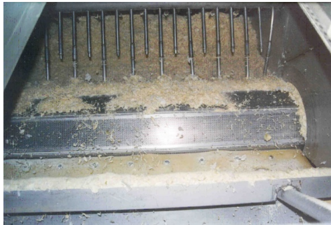
Figure 69. Photograph of the 3.8 m wide onion drying belt in Nevada, USA (site visit Lund, 1994).
