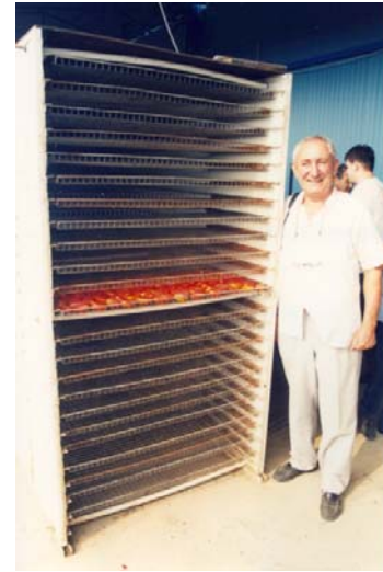
Figure 61. Drying racks used in the Greek tunnel drier (Andritsos, et al., 2003).
