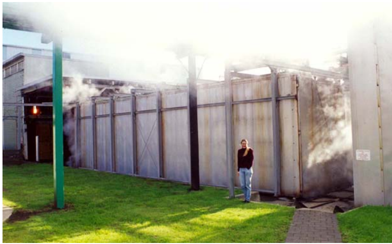
Figure 80. Lumber being dried with geothermal steam in closed kiln (Kawerau, New Zealand). Note steam escape above the unit (Scott and Lund, 1998).
