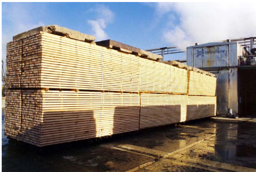
Figure 79. Lumber stacked prior to drying. Note the spaces between layers and the weights on top (Kawerau, New Zealand) (Scott and Lund, 1998).
