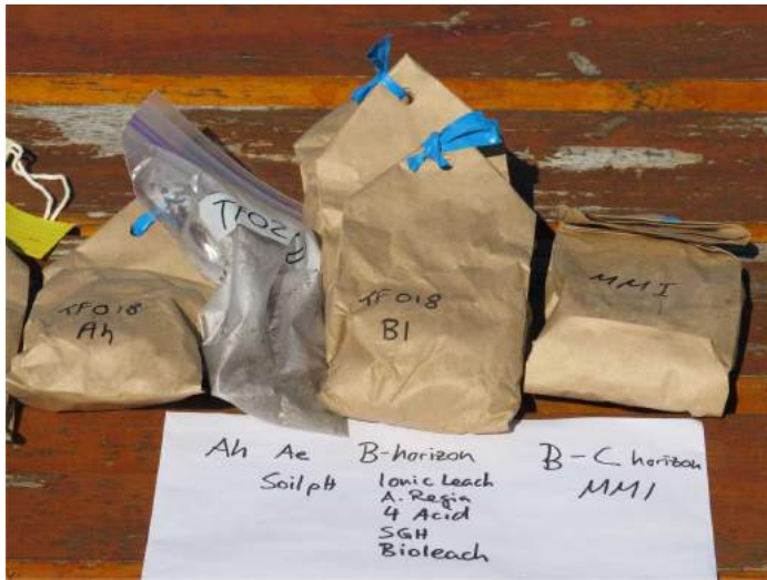
Figure 5. Suite of samples collected at each sample station for this study (not shown are spruce twigs and bark), Woodjam prospect, south-central British Columbia. The samples were collected together with those reported in Heberlein et al. (2013) and Ah results are discussed therein. MMI samples were not collected over basalt but results are briefly discussed in the appendix to this report.
