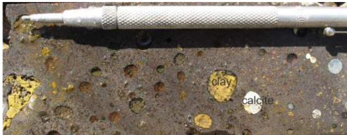
Figure 6. Example of vesicular Chilcotin basalt, with beige-brown clay (vermiculite) infill and white calcite infill, from drillhole MAG-12-04 (at 70.9 m) in the Three Firs zone, Woodjam prospect, south-central British Columbia. These two types of infill have been separated and analyzed by inductively coupled plasma-mass spectrometry (ICP-MS) following an aqua regia digestion to test for a geochemical signature from underlying mineralization.
