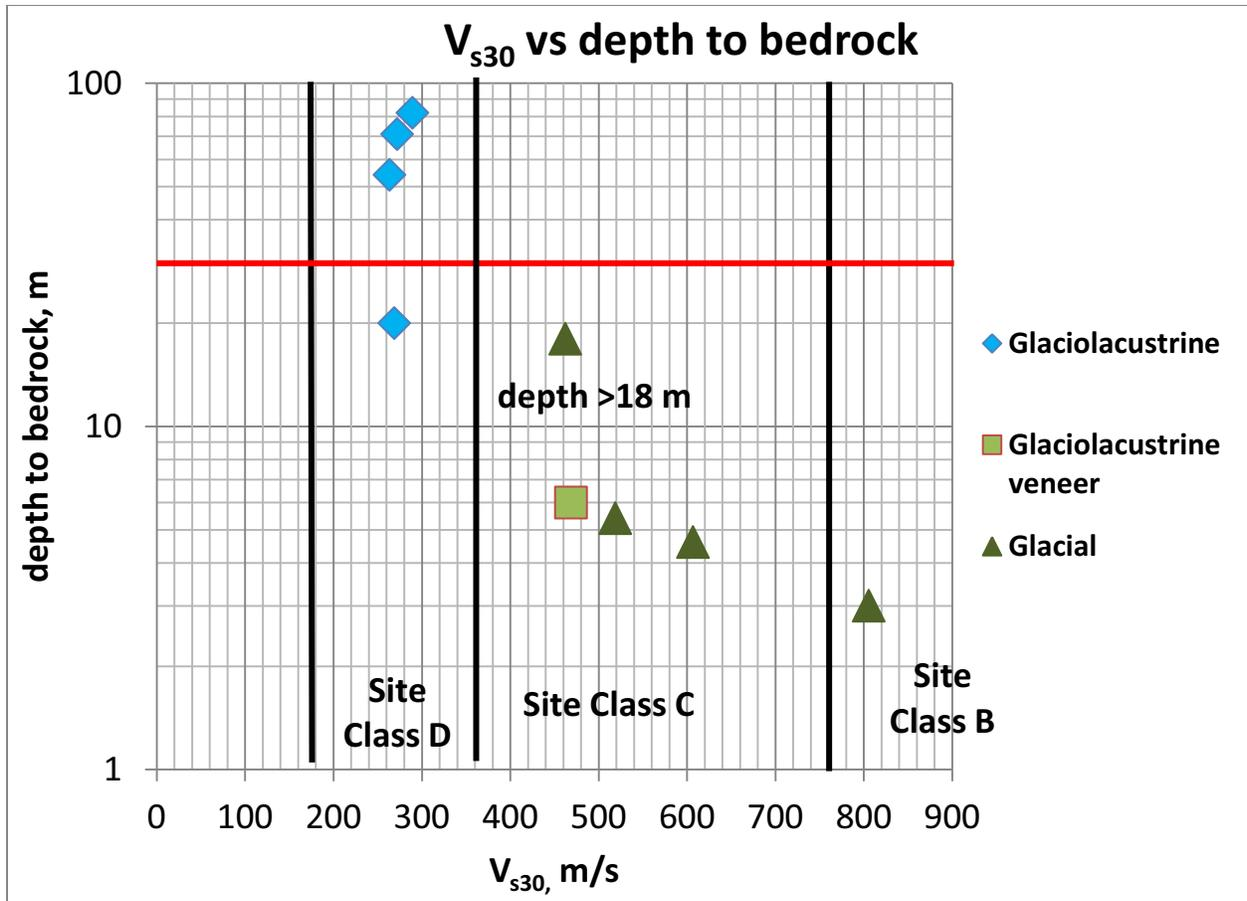
**Figure 13.** Depth to bedrock vs.  $V_{s30}$  for  $V_s$  sites where depth is known from borehole data. Note that the south end of SL2-6 where the depth is >18 m is added to complement the description of the Glacial map unit. Note also the red line that marks depth of 30 m, beyond which bedrock  $V_s$  does not contribute to  $V_{s30}$ .
