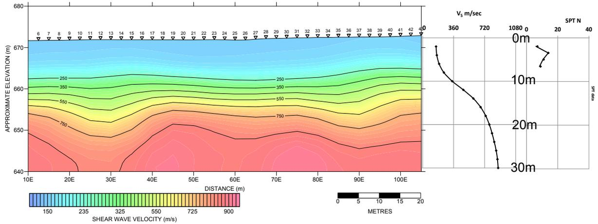
Figure 10a. Multichannel analysis of surface waves (MASW) profile for site SL-2, 94<sup>th</sup> Avenue, Fort St. John.  $V_{s30}$  is  $344 \pm 14$ , Site Class-D (Table 5). The borehole near east end (right) of line penetrated 7 m of glaciolacustrine silt with SPT  $N < 15$ .  $V_s$  panel right of profile is the trace at a single geophone. Note low velocities in the upper ~10 m. Note that  $V_s$  levels off at high value at base of profile, indicating unweathered bedrock.
