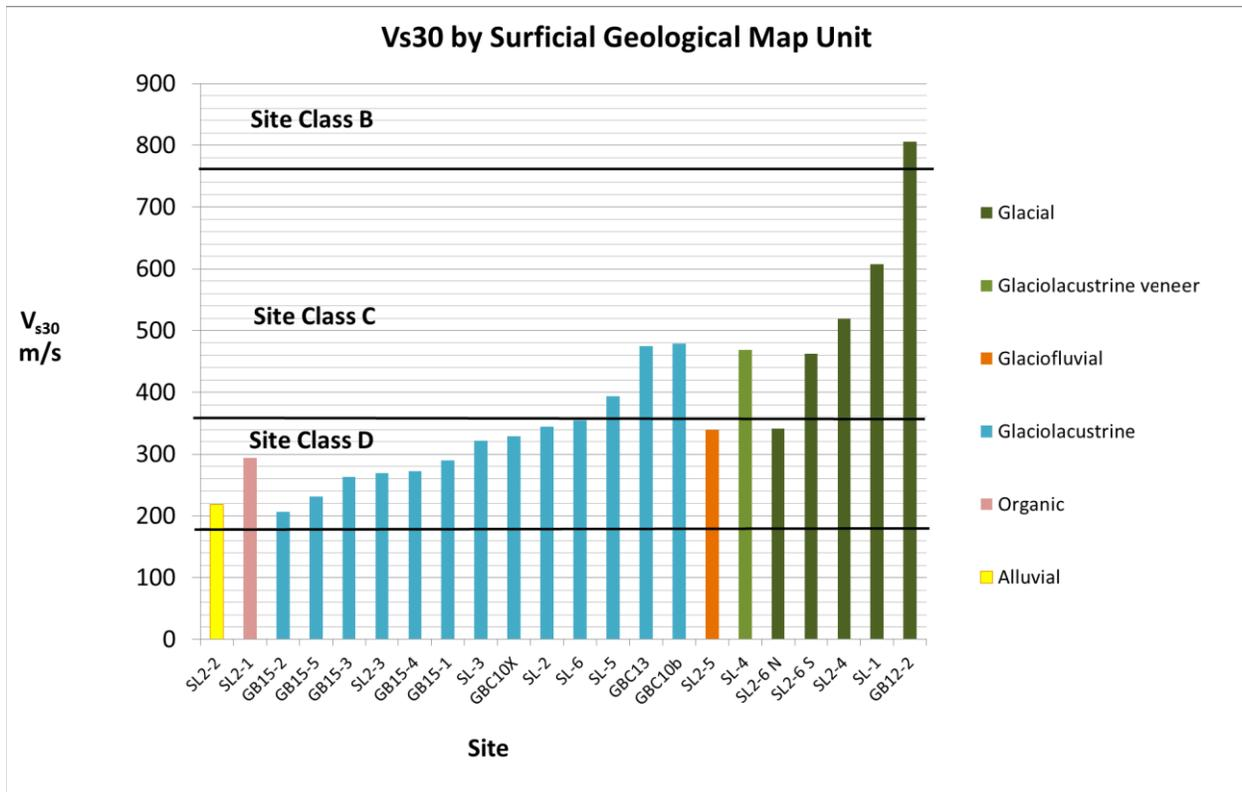
**Figure 12.**  $V_{s30}$  by surficial geological map unit. Note that MASW site SL2-6 is represented twice, because the geological profile at the south end, adjacent to the geotechnical boreholes, is significantly different than at the north end.
