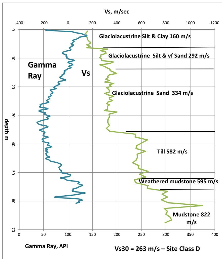
**Figure 9.** Shear-wave velocity ( $V_s$ ) and gamma-ray logs from borehole GB15-3 at Groundbirch, northeast British Columbia. Gamma-ray data from Weatherford, in Hickin *et al.* (2016a). Abbreviation: vf, very fine;  $V_{s30}$ , average shear-wave velocity in the upper 30 m.
