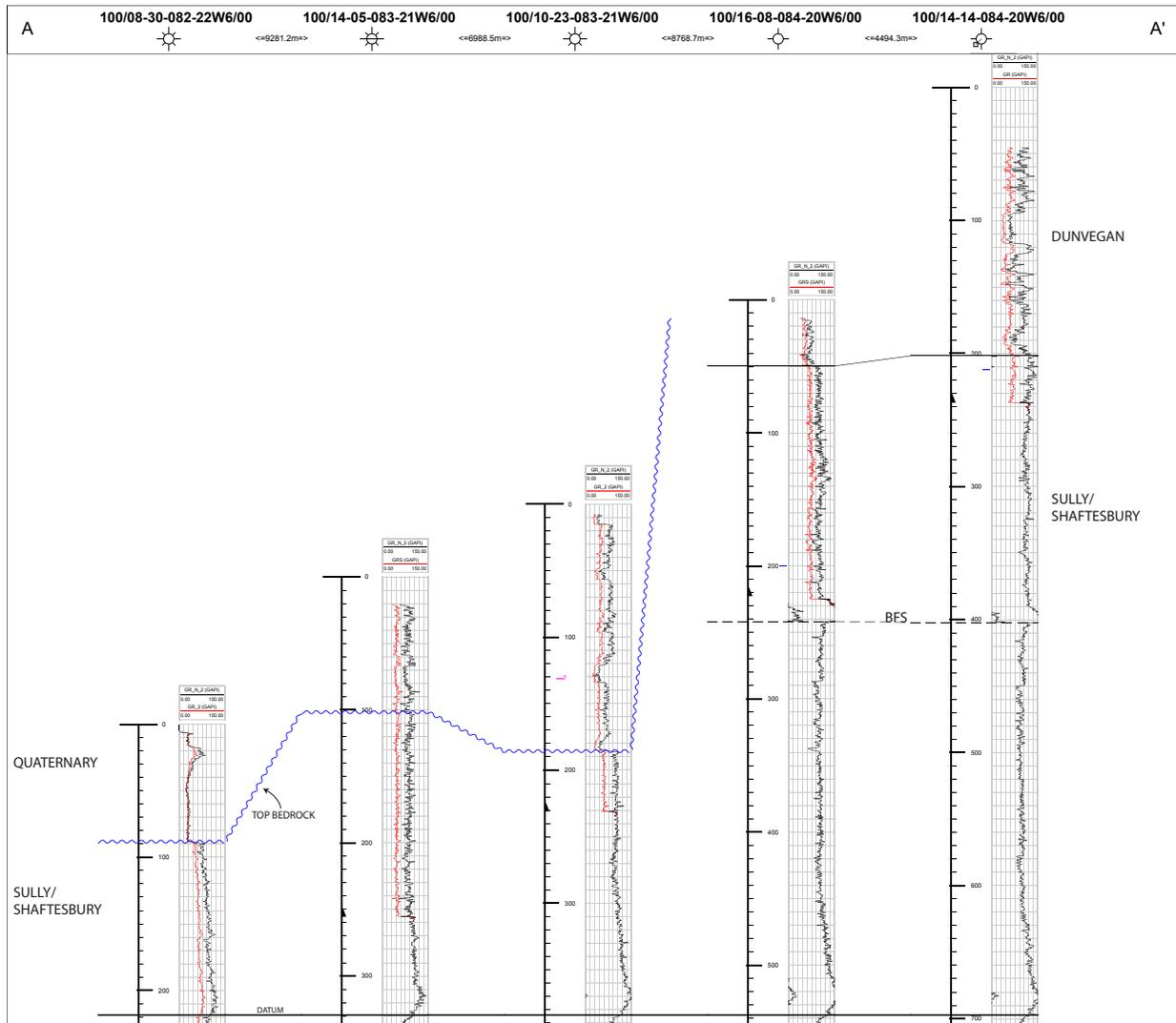
Figure 7a. Gamma ray log cross section, showing the high correlatability of the Cretaceous shales and the identification of thick Quaternary sediments in the southwest part of the cross section. Note in two wells on the right the log does not go to surface, so only a maximum depth to bedrock could be determined. Note the red curve is the originally recorded gamma ray signal behind surface casing, and the adjacent black curve is the corrected curve.
