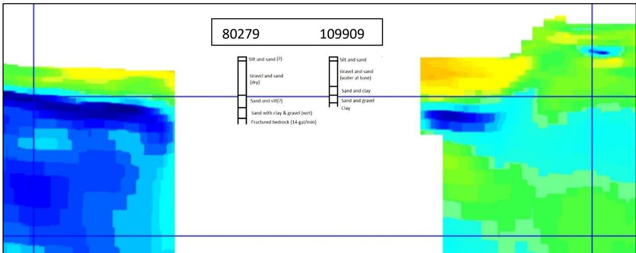
Figure 7. Lithology logs for water wells 80279 (left) and 109909 (right) plotted on EM cross-section L117202N.
