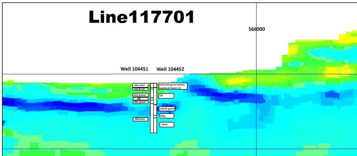
Figure 8. Lithologic logs for water wells 104451 and 104452 plotted on EM Line 117701
