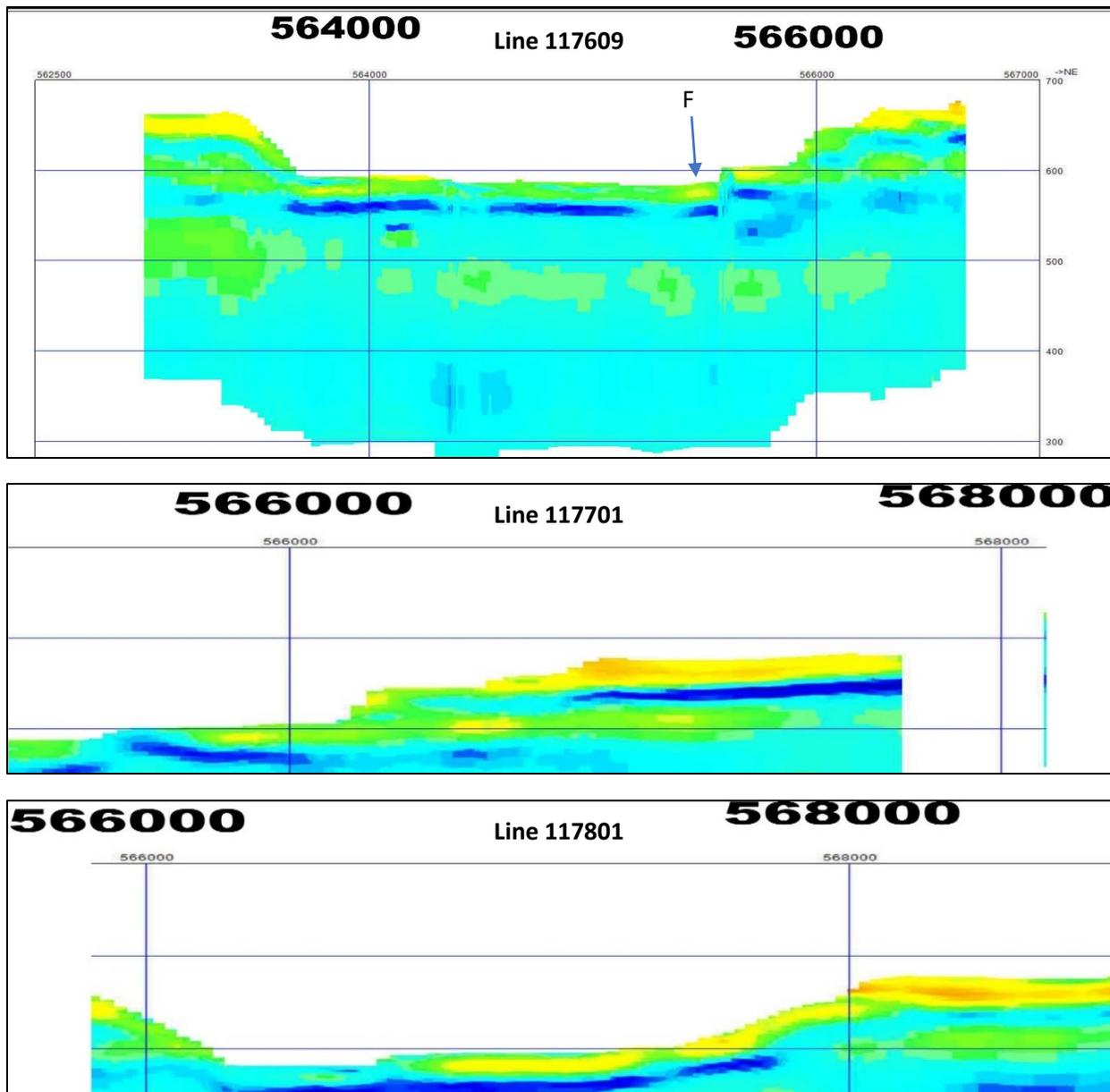
Figure 14. Northeast-trending EM sections in the southeast part of the study area: Benches east of the HRFN community are shown on the right side of each figure; view towards the northwest; vertical scale on all figures is about 1:5000 (2 cm = 100 m); horizontal scales shown
