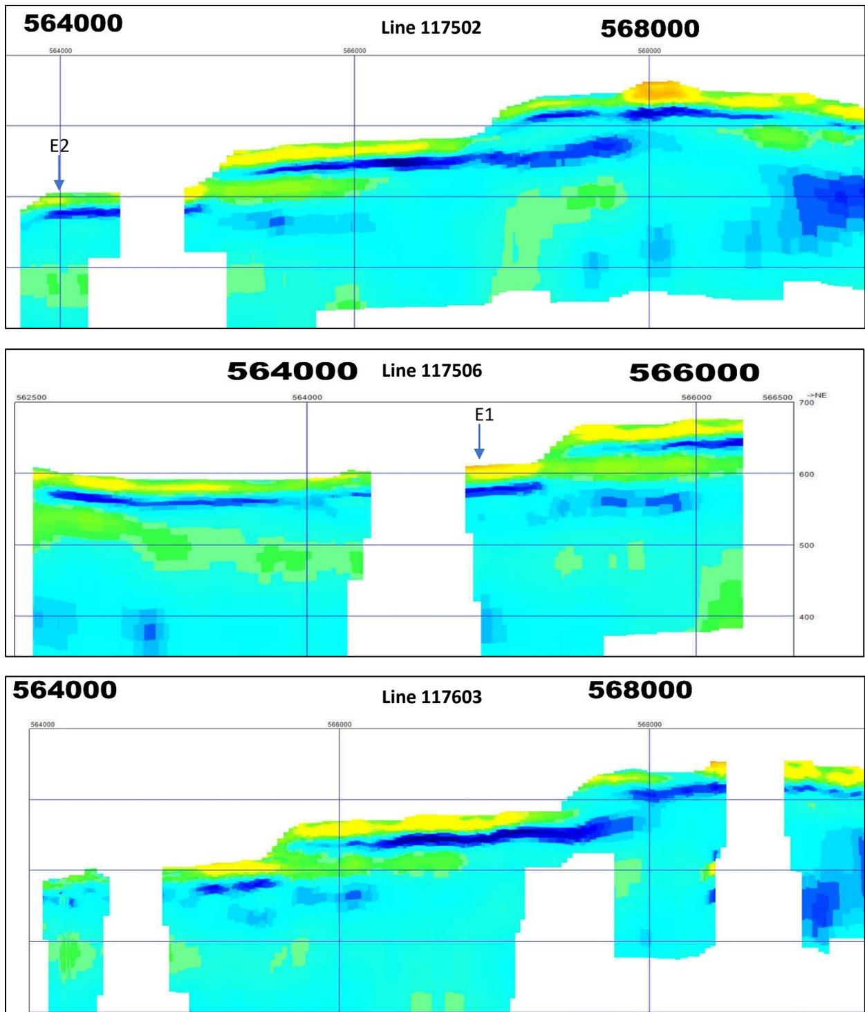
Figure 13. Northeast-trending EM sections in the central part of the study area: Upland areas and high glaciofluvial benches east of the HRFN community are shown on the right side of the figure; view towards the northwest; vertical scale on all sections is about 1:5000 (2 cm = 100 m); horizontal scales shown
