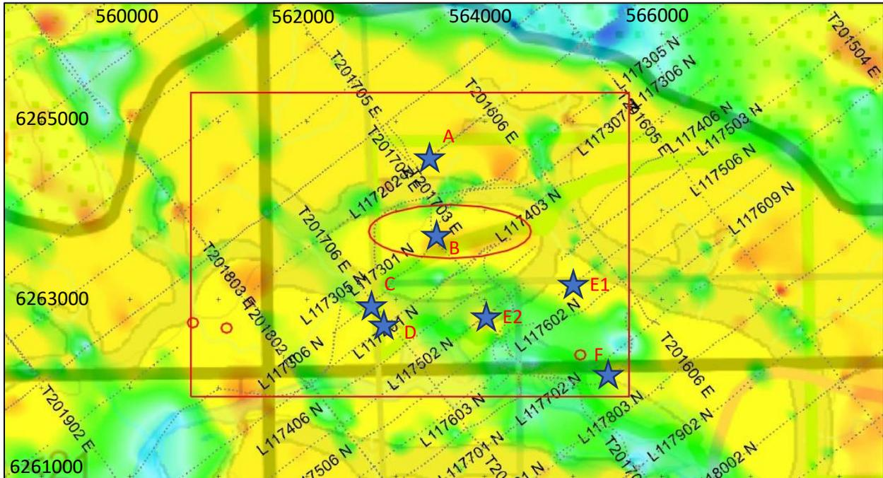
Figure 6. Location of EM flight lines overlain on the 10-15 m EM depth slice. The red circle outlines the area of the HRFN community and the red box outlines the primary study area. UTM easting and northing coordinates are shown on the top and left sides of the figure, respectively. Stars show target water well locations A to F.
