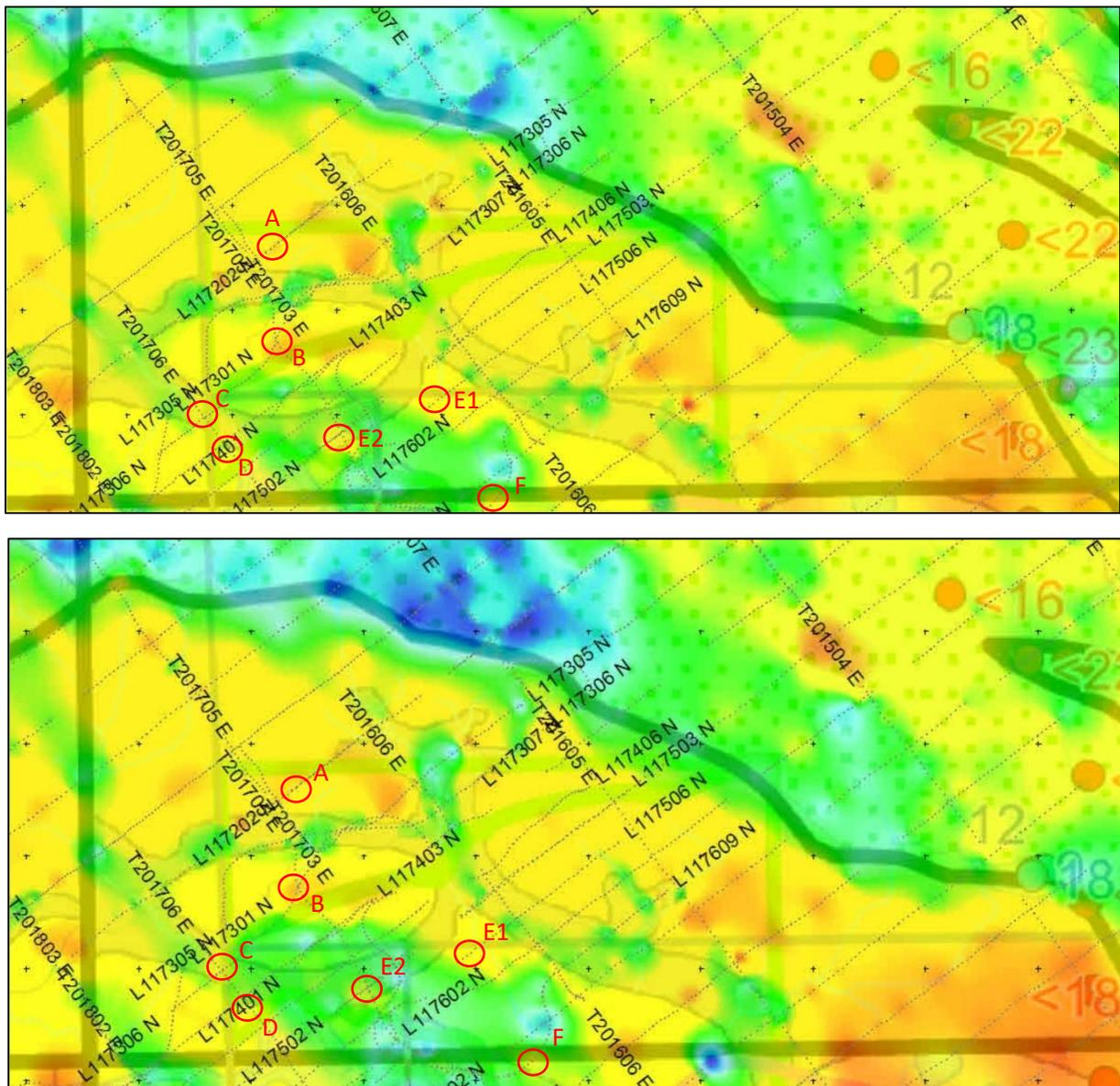
Figure 16. EM resistivity depth slices in the study area (top: 10-15 m; bottom 15-20 m) area and proposed drill targets (A-F)
