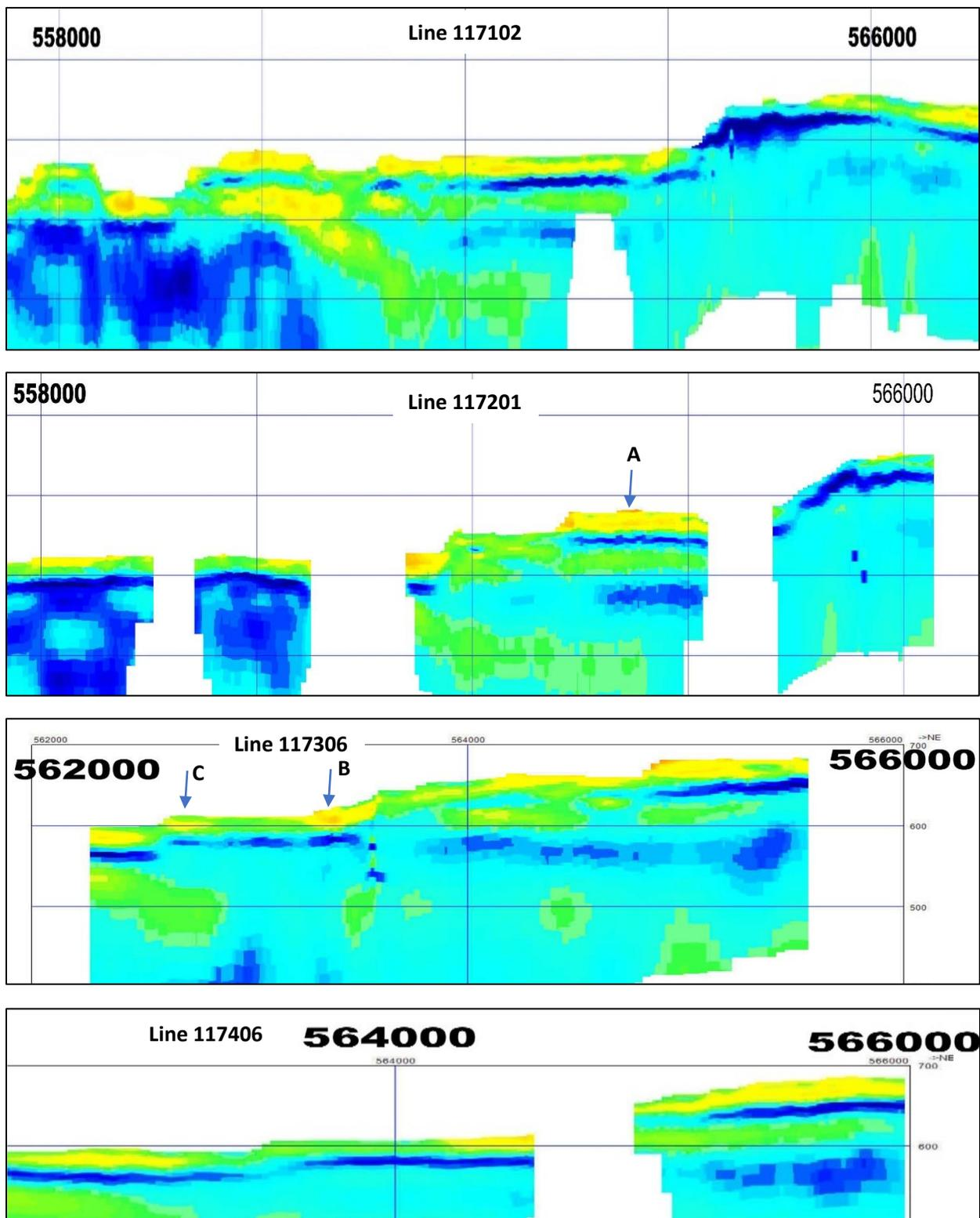
Figure 12. Northeast-trending EM sections in the northwest part of the study area: High bench northeast of the HRFN community is shown on the right side of each figure; view towards the northwest; vertical scale on all figures is about 1:5000 (2 cm = 100 m); horizontal scales shown.
