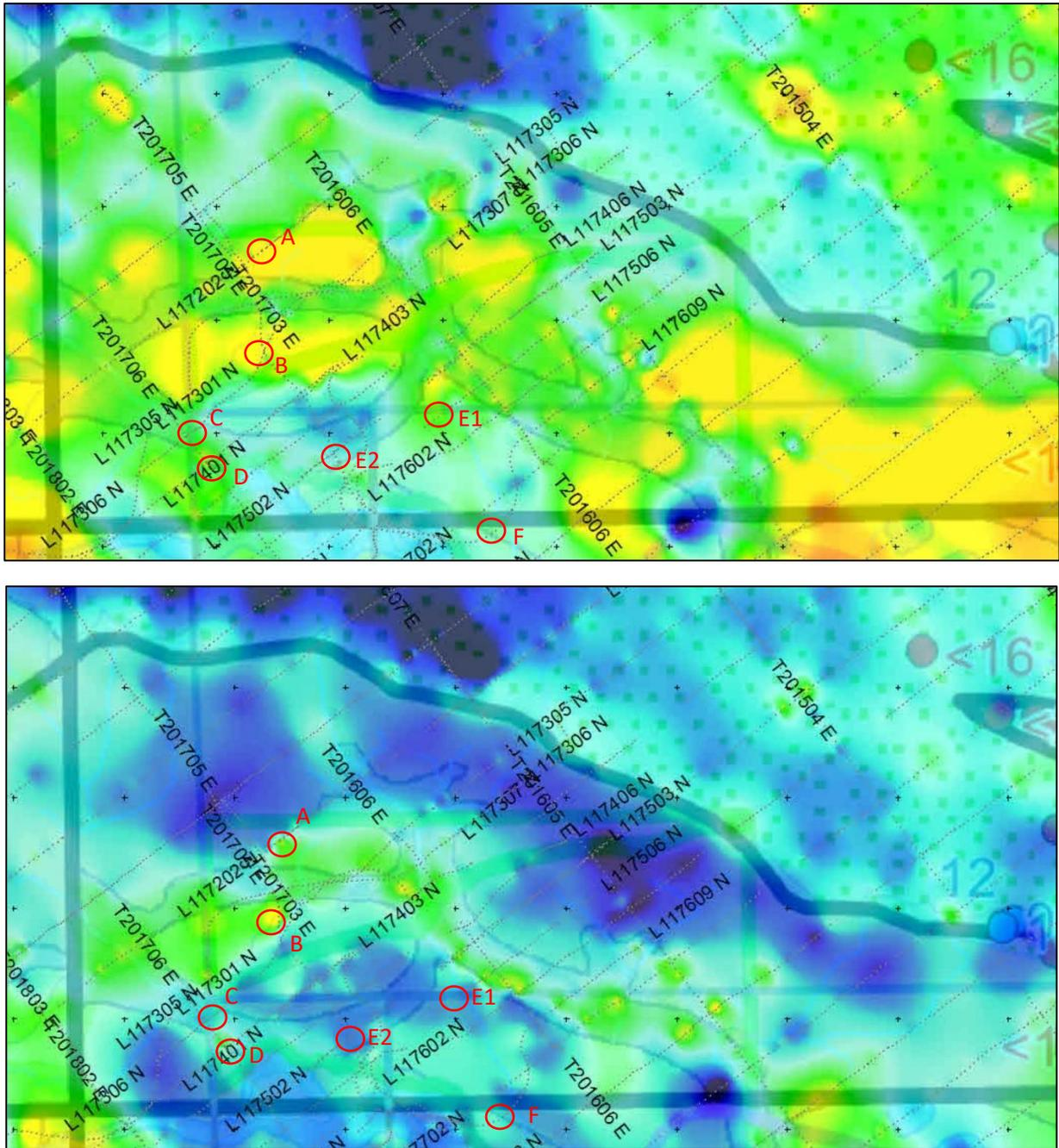
Figure 17. EM resistivity depth slices in the study area (top: 20-30 m; bottom 30-40 m) area and proposed drill targets (A-F)
