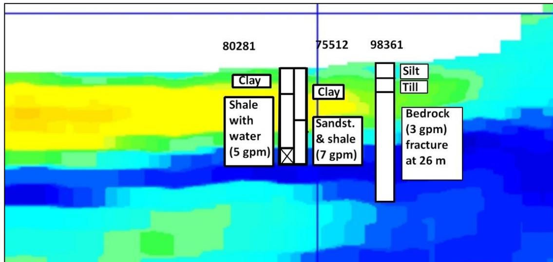
Figure 10. Lithologic logs for water wells 80281, 75512 and 98361 plotted on EM Line 118001.
