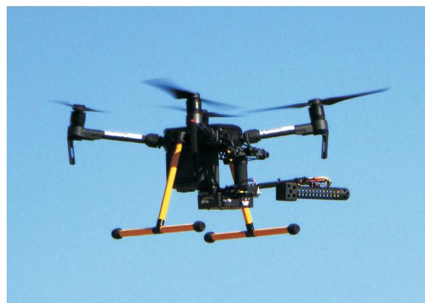
**Figure 1.** GHGMap's open-path laser spectrometer (OPLS) on a small unmanned aerial vehicle (UAV).
