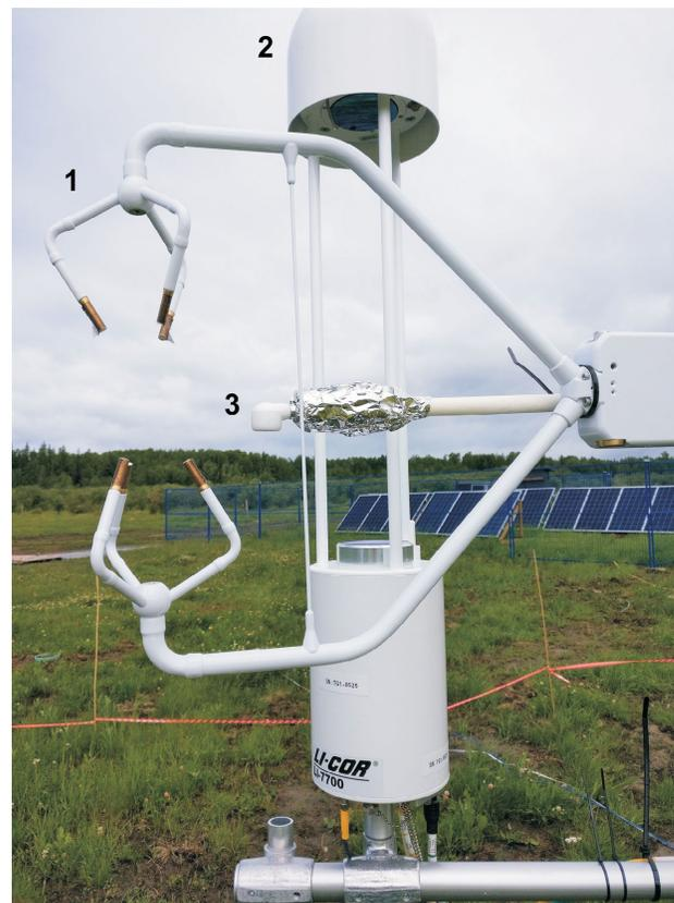
**Figure 10.** The instruments shown are the 1) sonic anemometer (CSAT3B, Campbell Scientific, Inc.), 2) open-path methane analyzer (LI-7700, LI-COR, Inc.), and 3) air sampling tube connected to the enclosed infrared gas analyzer for carbon dioxide and water vapour (LI-7200, LI-COR, Inc.).
