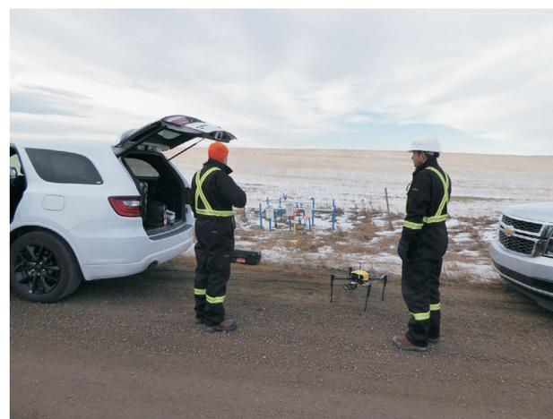
**Figure 10.** Photograph of open-path laser spectrometer/unmanned aerial vehicle (OPLS/UAV) platform at location 01 survey site, at AltaGas Utilities Inc., Alberta.
