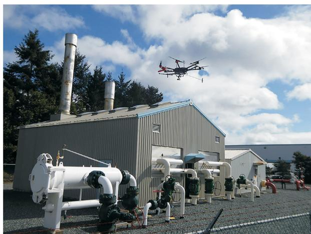
**Figure 2.** GHGMap's open-path laser spectrometer/unmanned aerial vehicle (OPLS/UAV) platform surveying at a gas distribution plant, Victoria region, British Columbia.
