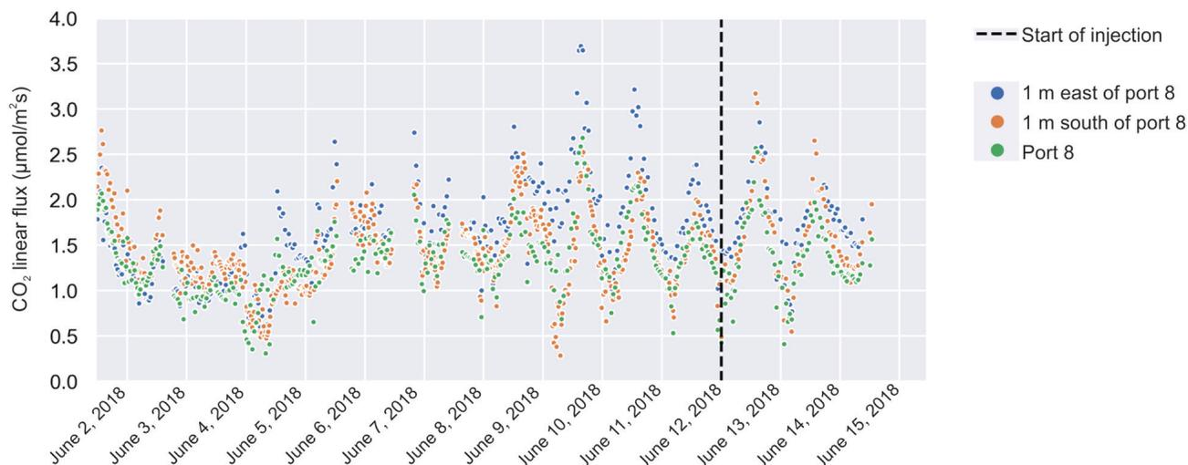
**Figure 8.** Example of carbon dioxide fluxes as measured from the long-term dynamic chambers, saturated zone site, northeastern British Columbia. It shows natural fluctuation before and shortly after injection (June 12) commenced.
