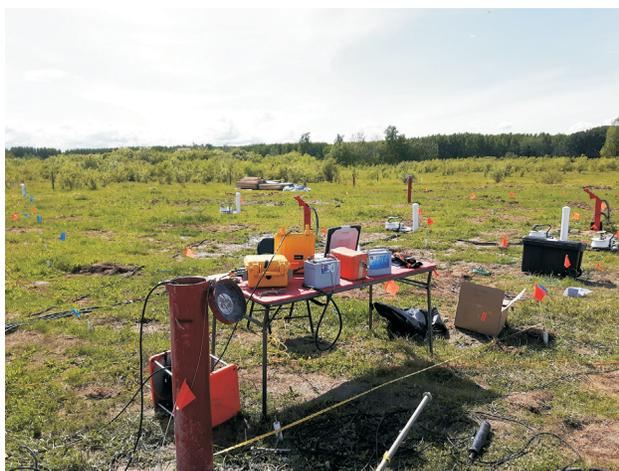
**Figure 6.** Vertical seismic profile set-up, saturated zone site, northeastern British Columbia.
