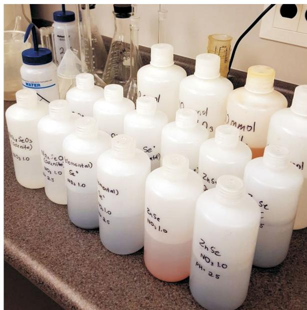
**Figure 2.** Selection of batch reactors used to evaluate Se oxidation.
