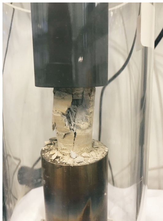
Figure 1. A tailings cylinder after being compressed until failure. The sample was cemented by the formation of secondary magnesium-carbonate minerals after exposure to a 10% \text{CO}_2 gas stream for three weeks.
