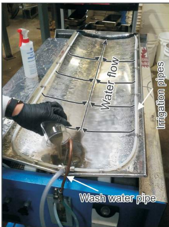
Figure 4. A sample being poured onto a Mozley C800 laboratory mineral separator. Water is supplied to the v-profile tray by the wash water pipe (copper tube) and the irrigation pipes (two white plastic tubes with water outlets at regular intervals). The direction of water flow is denoted by black arrows.
